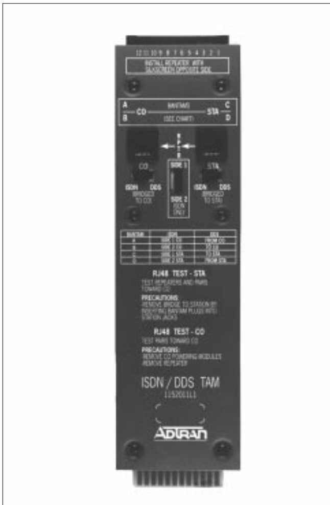
Figure 3. ISDN/DDS Test Access Module
