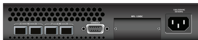
Figure 6. NetVanta 1534 Rear Panel Layout
